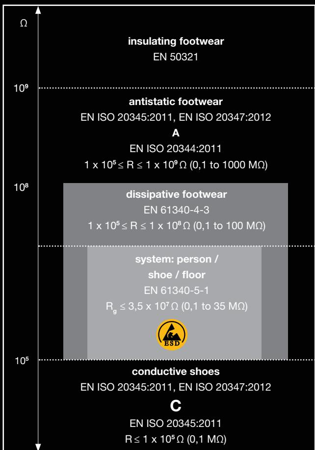
A and C: additional requirements of occupational- and safety shoes regarding electric property. R: electrical resistance.  $R_g$ : ground resistance.
